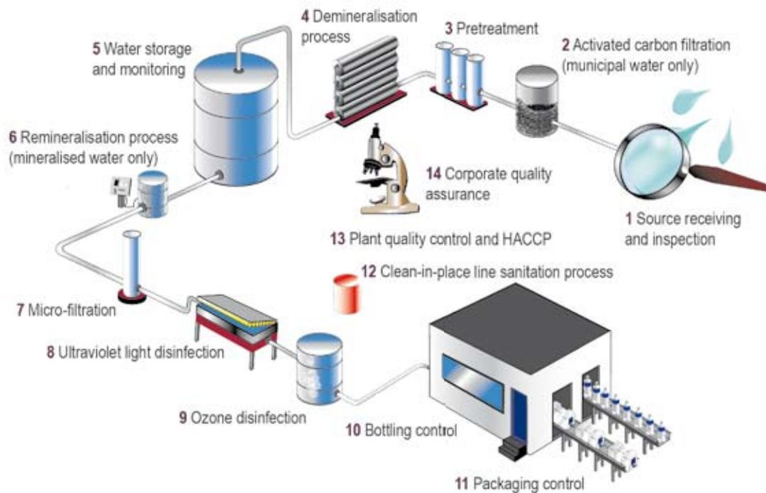
1. Water is carefully collected and received through stainless steel pipes from either a local well or municipal water supply. Quality testing of the original source is conducted regularly to monitor for abnormalities.
