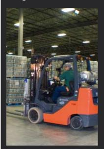
In 2005, gasoline-fuelled forklifts at the ECO DE LOS ANDES plant in Argentina were replaced with LPG (liquefied petroleum gas) forklifts in an effort to reduce emissions. Our successful reduction of these gases includes CO, HC, NOx, lead,  $C_xH_x$  and particulates.
