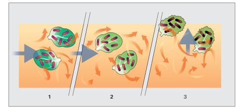
When considering a drying process with a continous reduction of product moisture, the inactivation of microorganisms is more likely to take place in the initial part of the process, when the target product temperature is reached and before the moisture level becomes too low for any inactivation to happen. The present booklet focuses on this part of the drying process.
