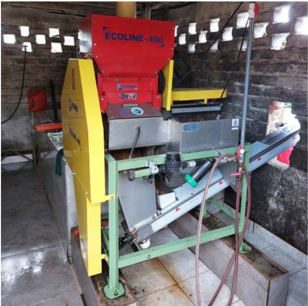
☞ A coffee wet mill that combines three processing steps in a single machine and significantly reduces water consumption compared to conventional wet processing: The ripe coffee cherries are pulped and classified without water. The pulped coffee is then directed to the demucilating process with low water consumption (0.2 l/kg of cherries). A screw conveyor transports and mixes pulp and mucilage without water. The machine also measures water consumption (Colombia) | CIAT/M. Pulleman.
