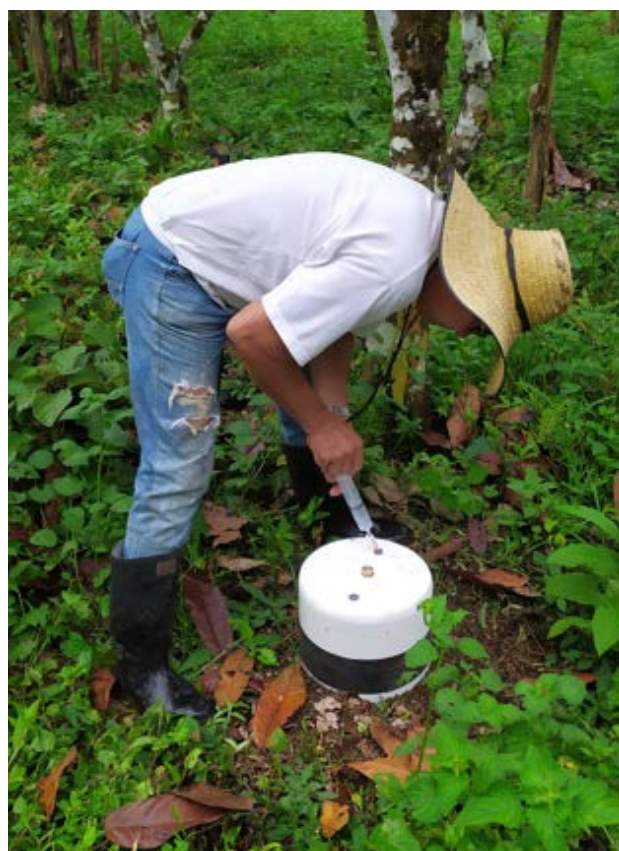
Taking gas samples in the field for the measurement of GHG emissions from soil | CIAT/M. Romero.
