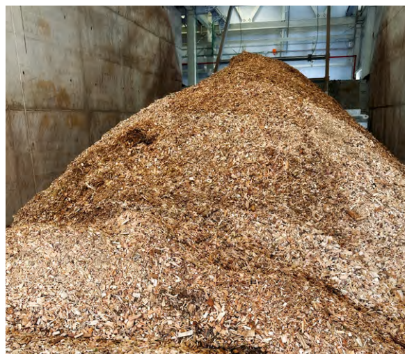
Wood chips sourced from forest-thinning operations are blended with spent coffee grounds to power Nestlé's Girona factory through two biomass boilers.
