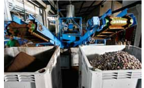
RECYCLING: Aluminium is separated from the coffee grounds of returned, used Nespresso capsules at a recycling centre.
